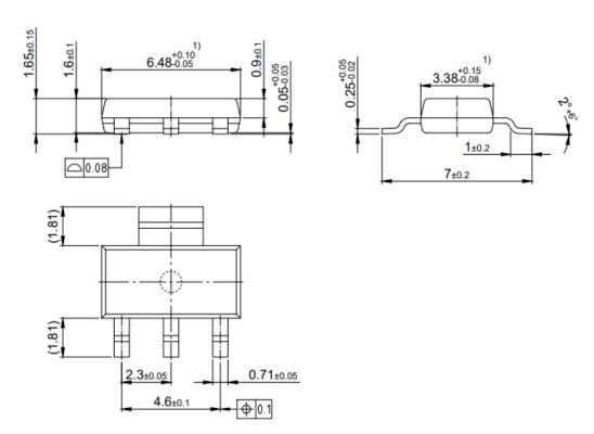
1) All dimensions refer to JEDEC standard TO261-AA do not include mold flash or protrusions, body length including mold protrusions shall not exceed 6.7mm.
